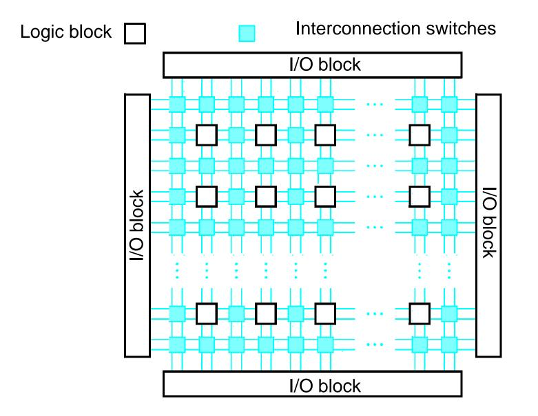
Structure of an FPGA
